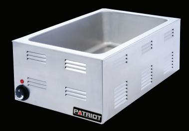
Patriot's full size food warmer is constructed with a stainless steel housing for excellent durability. The interior well is constructed of 20 gauge 18/8 stainless steel with a 10" x 20" opening that is 6.5" deep to accommodate all standard size food pans up to 4" deep. The dual element design provides efficient and even heat distribution. This item maintains food temperature at HAACP standards of 140°F-145°F.
